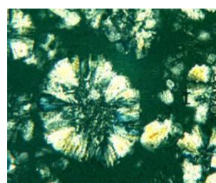
Pseudo-Radial Structure or Morphology: Crystal growth on small to medium sized particles with Mosaic Structure results in hydrate particles with Pseudo-Radial Structure and medium concentration of grain boundaries.
