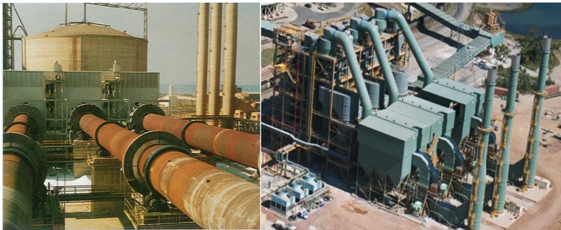
Figure 1. 3xØ 3.95 x 107 m rotary kilns 3 x 4500TPD GSC units with bag filters.
